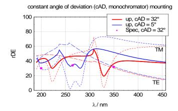
Typical efficiency curves based on rigorous electromagnetic modeling using measured AFM profiles. rDE refers to the ratio between diffracted power from the grating and reflected power from a mirror coated with the same material.
